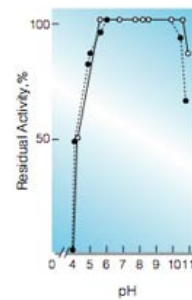
Fig.4. pH-Stability [25°C, 20hr-treatment with 50mM buffer solution: pH4.0-6.0, acetate; pH6.0-8.5, phosphate; pH9.0-11.0, carbonate: ○ — with 0.01% mercaptoethanol ● — without mercaptoethanol
